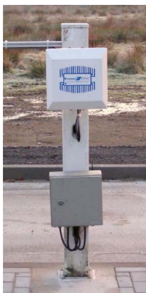
Tower with antenna and central unit in weatherproof housing
