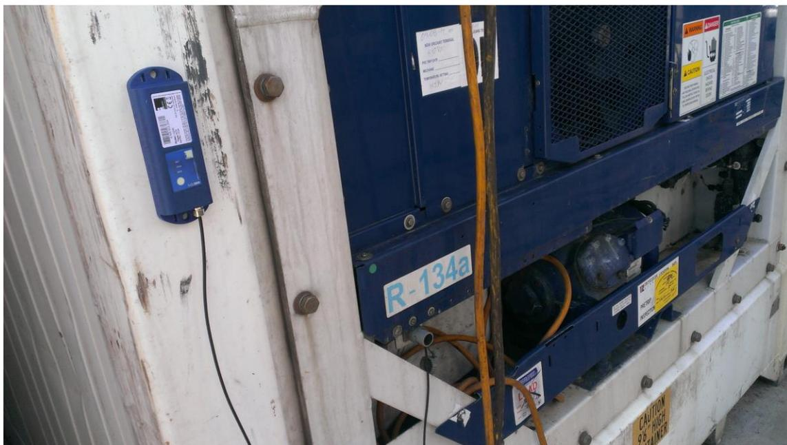
© IDENTEC SOLUTIONS A magnetically fixed tag produces an automatic link with the container's controller
